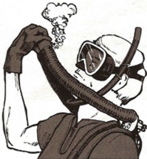
Fig. 1-93 Purging the Double Hose Regulator
